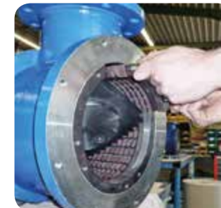
Simply by modifying the ROTOR and STATOR in the housing, particle sizes can be varied from 0,3 mm to 20 mm.
