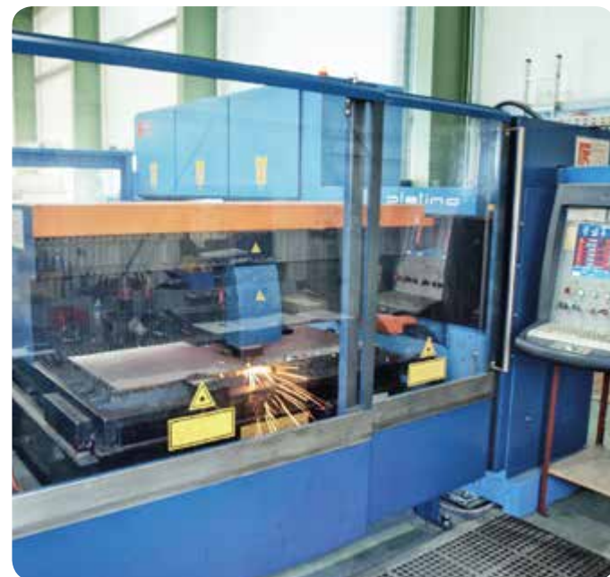
Laser for large format (3 x 1.5 m) with a thickness of up to 20 mm. Edging up to 3 m and thickness of 8 mm
